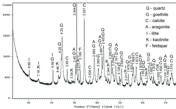
Fig. 7. X-ray diffraction pattern of minerals in the most external part of weathering crust
