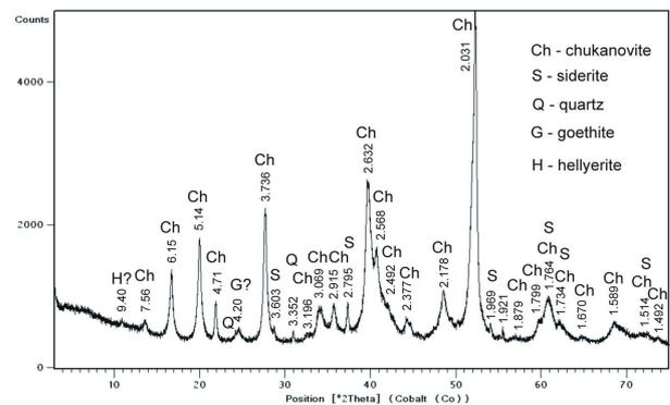
**Fig. 10.** X-ray diffraction pattern of chukanovite
