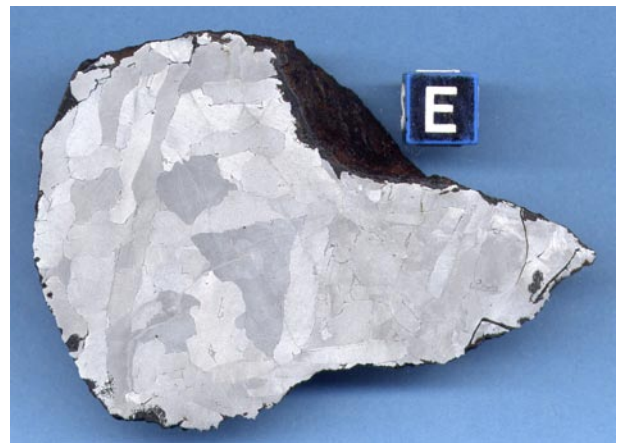
Fig. 2. Etched cross section of the 544 g find
