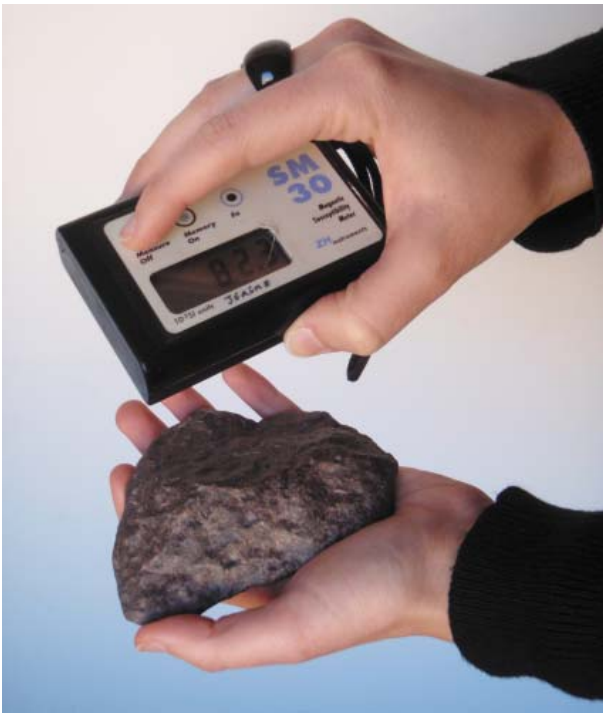
Fig. 1. Picture of SM30 while performing the “air” measurement on a large meteorite find from Atacama. \log \chi value is obtained by subtracting this air measurement from the one obtained at contact with the meteorite, and modeling the geometric correction following Gattacceca et al. (2004), using mass and bulk density. This geometric correction is required by the non-uniform field generated by the SM30 coil. In standard coils where the sample is inserted in a zone of uniform field inside the coil, this correction is not necessary, thus explaining the lower accuracy of SM30
