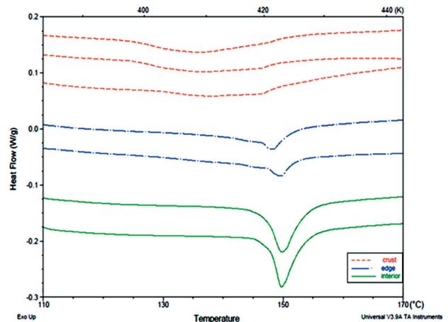
**Fig. 4.** Endothermic peaks of  $\alpha/\beta$  transition of troilite from different parts of the NWA 6255 meteorite. DSC scan showing the heat flow during heating of the meteorite samples (dash line – crust, dash dot line – edge, solid line – interior)
