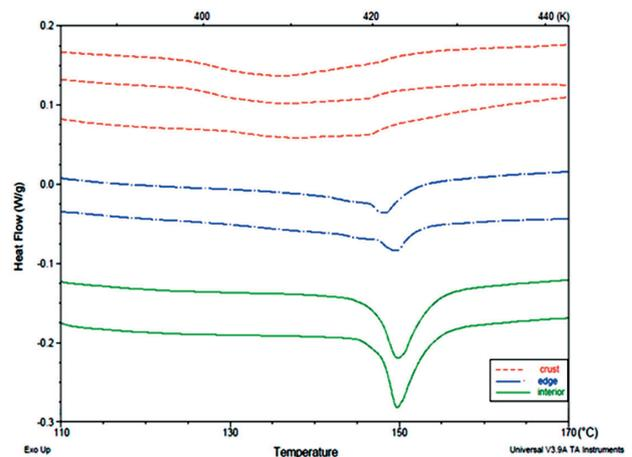
Fig. 4. Endothermic peaks of  $\alpha/\beta$  transition of troilite from different parts of the NWA 6255 meteorite. DSC scan showing the heat flow during heating of the meteorite samples (dash line – crust, dash dot line – edge, solid line – interior)
